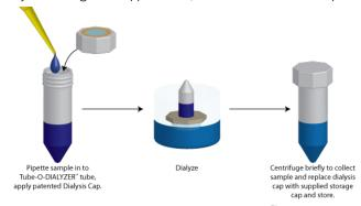
Figure 16: A summary of the Tube-O-DIALYZER™ system.
