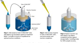
Figure 15: Tube-O-Reactor™ system.
