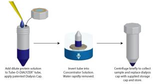
Figure 21: Tube-O-CONCENTRATOR™ scheme.
