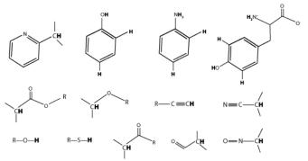
Figure 9: Active hydrogen containing compounds.
