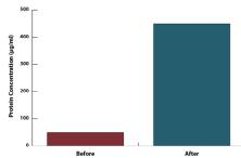
Figure 20: Column concentration of dilute proteins. 1ml dilute protein  $(50\mu g/ml)$  was concentrated with Column-PROTEIN-Concentrate<sup> $\infty$ </sup> to a final volume of 110 $\mu$ l with a concentration of 450 $\mu$ g/ml.
