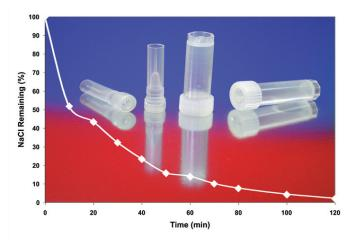
Figure 17: Tube-O-DIALYZER™ Micro (8K MWCO) Dialysis Rate. 100µl 5M sodium chloride was dialyzed against 1 liter deionized water. 50% sodium chloride is removed in the first 10 minutes.
