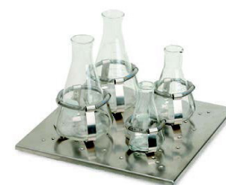
Flask clamp platform (Cat. No. S2031-18), clamps sold separately
