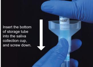
Anti-unscrew Storage Tube Cap Design:
