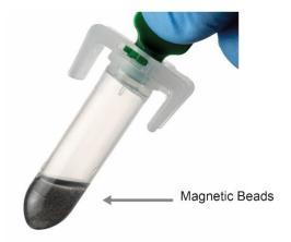
Magnetic Beads capture nucleic acids for transfer between steps.
