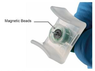
**4** Magnetic Beads are safely attached to SmartLid and ready for transfer into the next tube.
