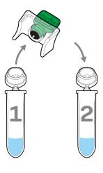
Transfer: Remove the SmartLid with collected Beads from tube 1 and place into tube 2.
