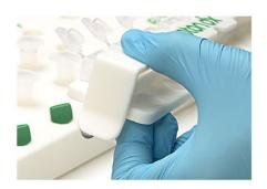
**Bead collection**: Inverting the SmartLid Shaker, with Magnetic Keys inserted, enables rapid and efficient Magnetic Bead collection.
