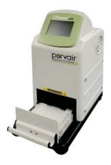
The Ultraseal LITE is a semi-automated heat-applied microplate and tube rack sealer. The unit uses pre-cut sheets of surface modified aluminum or plastic film, approximately 78mm wide and 130mm in length, applied to the plate top surface to create a seal between plate and film.
