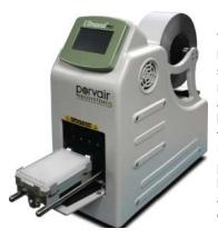
The Ultraseal PRO is an automated heat-applied microplate and tube rack sealer. The unit uses a roll of surface modified aluminum or plastic film, approximately 78mm wide and 610mm long. The roll is positioned to the rear of the sealing section via a removable stand. Using a total in-line method, the film is pulled through the main unit, cut to between 125mm and 130mm lengths, and applied to the plate top surface to create a seal between plate and film.
