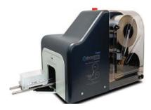
The Ultraseal coldPro automates the application of adhesive film to microplates and tube racks. The unit uses a roll of surface modified aluminum or plastic film, approximately 80 to 85mm wide and 200m long. The roll is positioned to the rear of the sealing section via a removable stand, using a total in-line method. The film is pulled through the main unit, cut to between 124mm and 130mm lengths and applied to the plate top surface to create a seal between plate and film.
