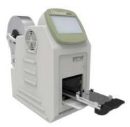
Featuring all-electric operation, the Ultraseal ePro removes the risk of cross-contamination inherent in compressed air powered sealers. The use of force-sensors allows dynamic feedback during the entire sealing process to ensure a complete homogenous seal. All operations are controlled through an intuitive touchscreen interface. Capable of handling foil lengths between 116mm and 128mm, the ePro automatically compensates for variations in plate heights.
