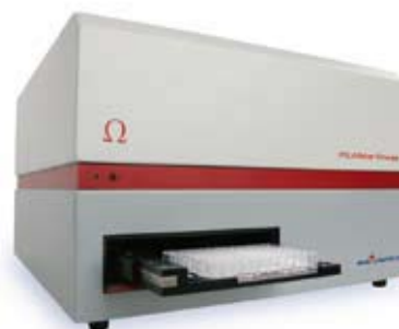
Fig. 2: BMG LABTECH's POLARstar Omega multidetection microplate reader.
