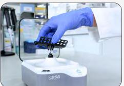
**Quick and Easy Rotor Change**To mount one of the two rotors, simply push it onto the drive shaft until there is an audible click. Remove it by pulling it straight up and off the shaft. **No tools required!**
