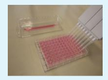
2 Incubate the plate for 1 to 4 hours in a humidified incubator
