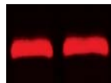
Figure 17: Visualization of TAMRA labeled BSA. 1µg (5/6) TAMRA-SE labeled BSA was resolved on a 4-20% SDS polyacrylamide gel.
