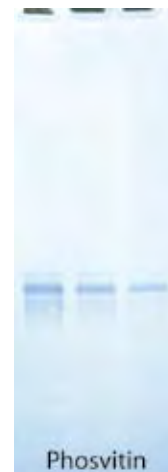
Figure 19: Various concentrations of phosphoprotein were loaded onto the FOCUS™ PhosphoRich™ columns and were washed extensively. The protein was rapidly eluted and the eluted proteins were resolved by SDS-PAGE. The phosvitin was visualized with the Reversible Zinc Stain™.
