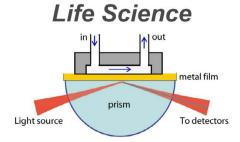
Our flow injection technology enables you to study biomolecular interactions and kinetics with greater resolution and precision, and is perfect for a diverse array of life science applications such as:
