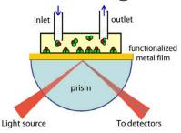
Unlike other SPR instruments, BI-SPR technology is capable of molecular binding analysis in gas phase. In addition to chemical vapor detection, our instruments facilitate sensor development, thin film characterization, and numerous other gas phase applications, which can help you study:
