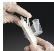
Clip top of funnel and base together.
