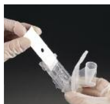
Place new filter onto microscope slide.
