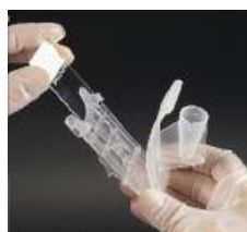
Insert microscope slide.
