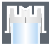
Loose position for aerobic work
